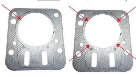
thickness allowed is .049". Measurement must be performed using a micrometer. Readings are taken from inside the cylinder hole of the gasket closest to the combustion chamber (see diagram). Four measurements must be taken with 3 meeting the minimum thickness of .049".
